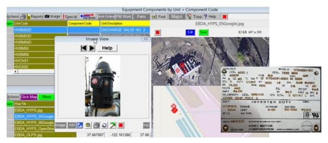
Nameplate information is also related to the equipment record. Nameplates can be scratched and overpainted in the future. Machine information on file is often incorrect when compared to nameplates.
